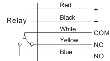
Fig. 8, 5A Relay output type wiring
