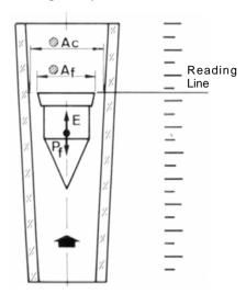
The flowmeter consists of a float inside a conical tube.
