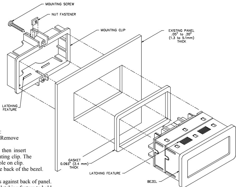
to approximately 75 to 80% of its original thickness. (Recommended torque is 28 to 36 in.-oz.)
